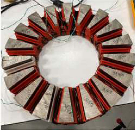
Figure 16. The DSSR-AFPM machine stator used as a torus test.
