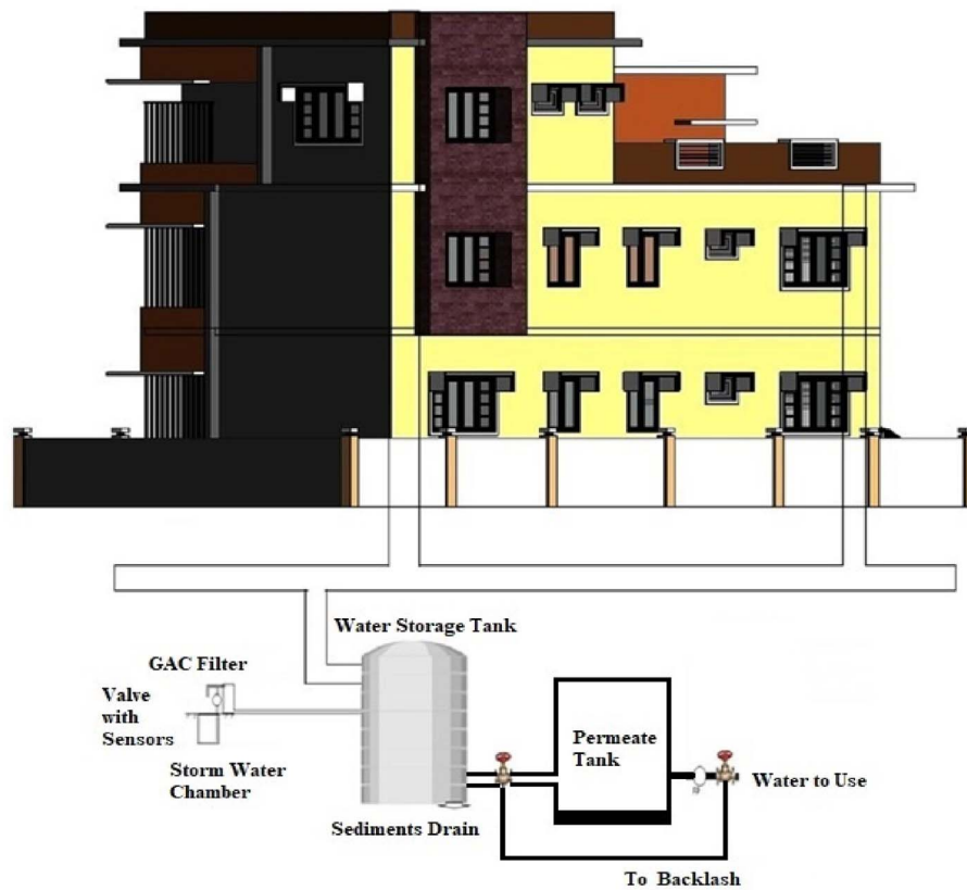
Fig. 9. Stormwater-harvesting system of proposed green building.
