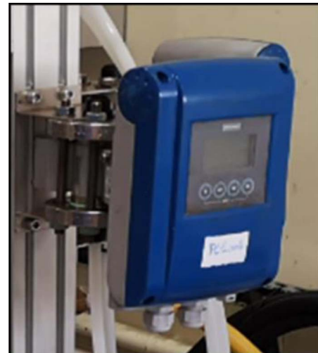
Figure 7. Electromagnetic mass flow meter Krohne Optiflux 4100.
