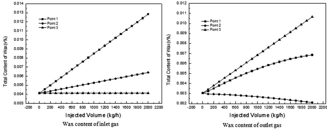
Fig. 12. The variation of wax content of inlet/outlet gas of high-pressure separator with the injected volume.
