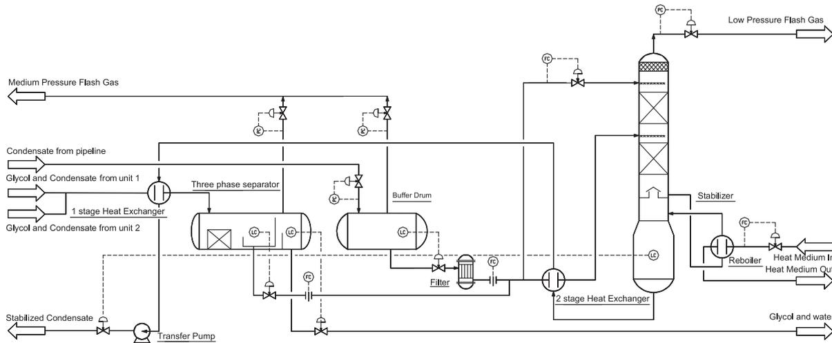
**Fig. 6.** The condensate stabilization unit flow diagram. Three-phase separator: Operation pressure: 1.5 MPa.g; Operation temperature: 50 °C; Buffer drum: Operation pressure: 1.0 MPa.g; Operation temperature: 50 °C; Stabilizer: Operation pressure: 0.4 MPa.g; Operation temperature: 140 °C (bottom of stabilizer), 83 °C (top of stabilizer).
