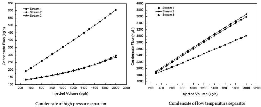
Fig. 10. The variation of condensate flow of high-pressure separator/low temperature separator with the injected volume.
