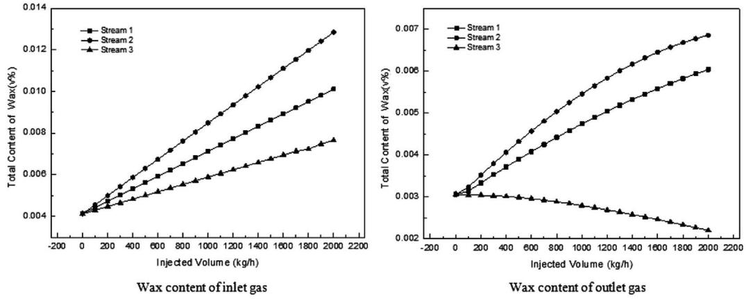
Fig. 9. The variation of wax content of inlet/outlet gas of high-pressure separator with the injected volume.
