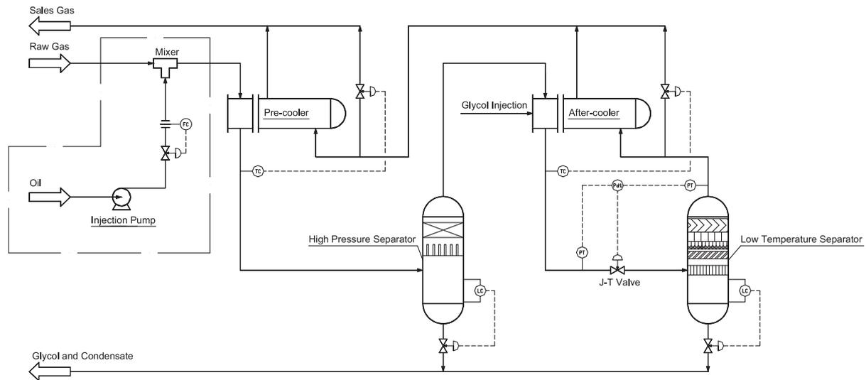
**Fig. 5.** Oiling Low Temperature Separation (LTS) process flow diagram. Pre-cooler: Operation pressure: 12 MPa.g; Operation temperature: inlet temp. 38 °C, outlet temp. 20 °C; After-cooler: Operation pressure: 11.9 MPa.g; Operation temperature: inlet temp. 20 °C, outlet temp. -10 °C; High pressure separator: Operation pressure: 12 MPa.g; Operation temperature: 20 °C; Low Temperature separator: Operation pressure: 7.9 MPa.g; Operation temperature: -26 °C.
