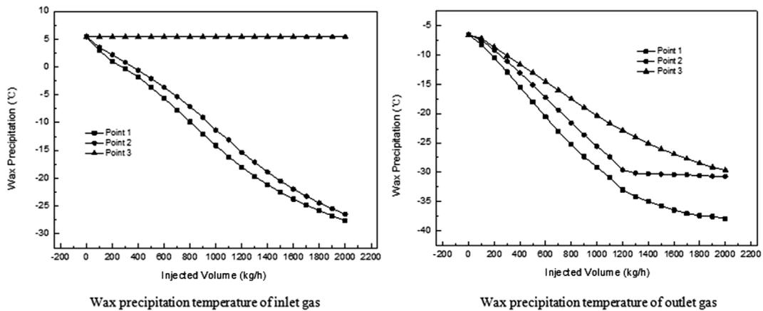
Fig. 11. The variation of wax precipitation temperature of the inlet/outlet gas of high-pressure separator with the injected volume.
