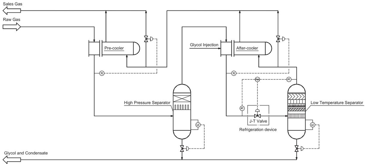
**Fig. 1.** Conventional Low Temperature Separation (LTS) process flow diagram. Note: J-T valve, expander and propane refrigeration system are used as refrigeration device for decrease the natural gas temperature.
