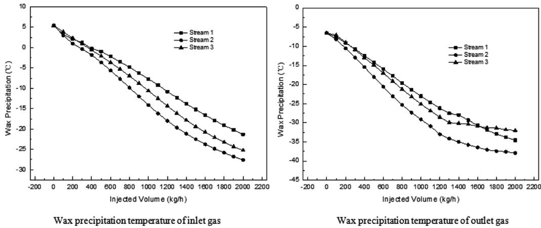
**Fig. 7.** The variation of wax precipitation temperature of the inlet/outlet gas of high-pressure separator with the injected volume.
