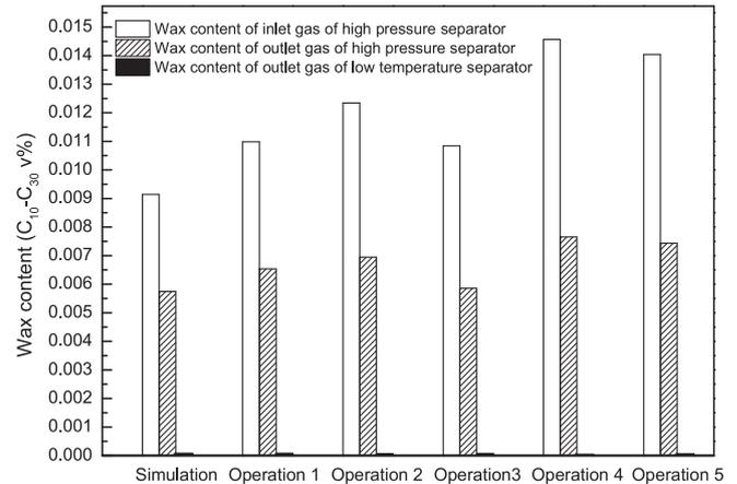
**Fig. 15.** The comparison of wax content between simulation and operation.
