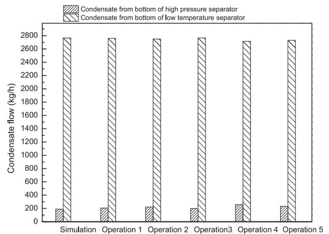
**Fig. 16.** The comparison of condensate between simulation and operation.
