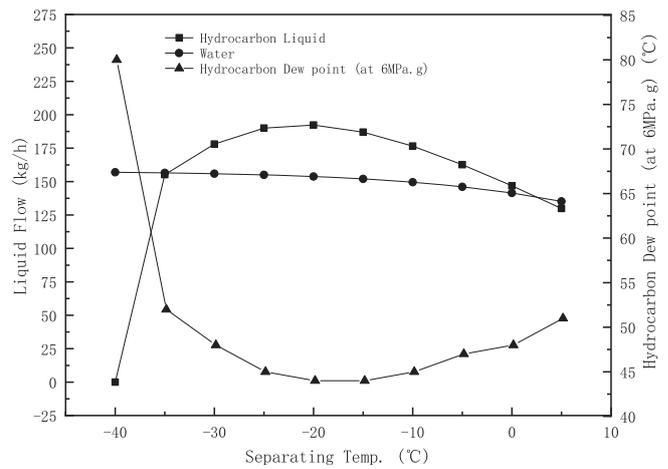
**Fig. 3.** Variation of heavy hydrocarbon liquid flow at different separating temperatures.
