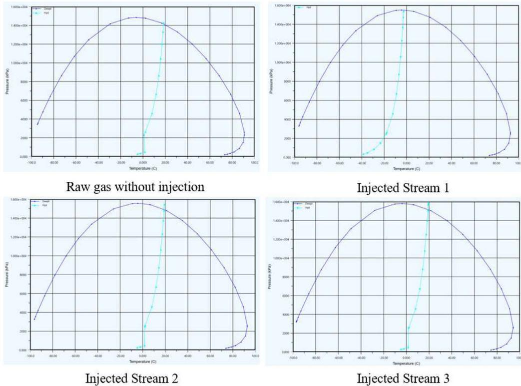
**Fig. 8.** The variation of gas-liquid equilibrium of raw gas with injecting stream.
