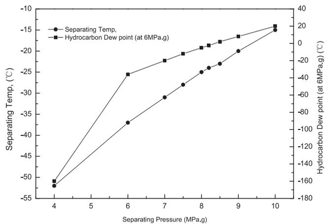
**Fig. 4.** The relation between the dew point and the separating (refrigeration) temperature.
